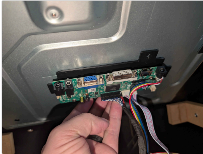
LVDS case mounting location.
