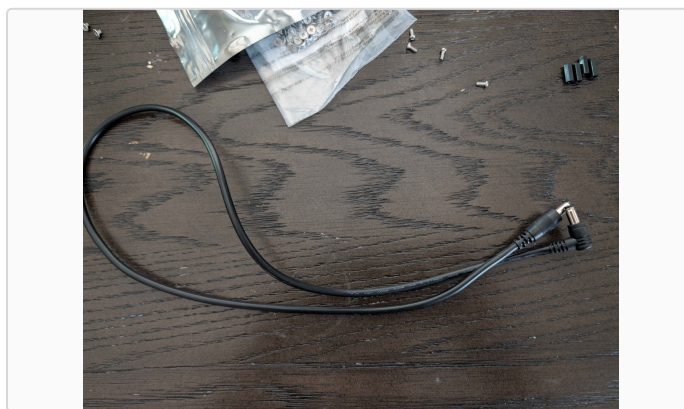
LVDS power cable (stock)
